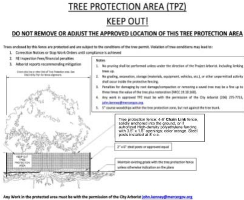
Image 3. An example of the required tree protection barrier signage.
